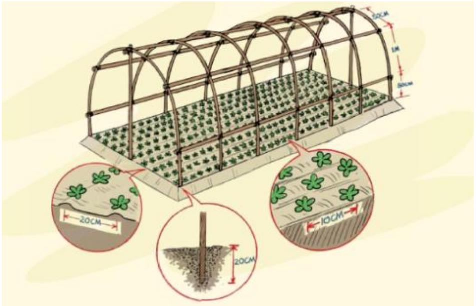
**Figure 6:** Details of net tunnel framework
