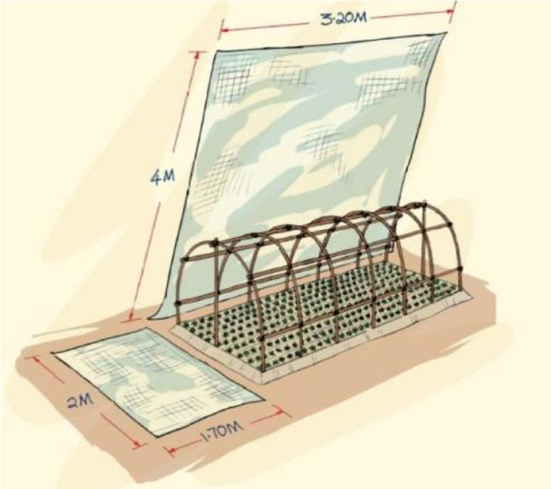
**Figure 7:** Details of net tunnel mesh
