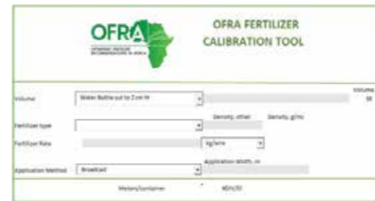
A fertilizer calibration tool is used to convert the recommendation, expressed as kg of fertilizer per hectare of land, to a more farmer-friendly measure.
