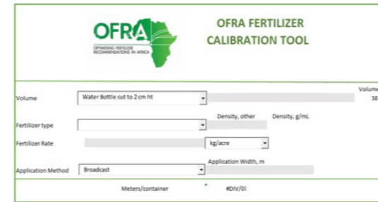
A fertilizer calibration tool is used to convert the recommendation, expressed as kg of fertilizer per hectare of land, to a more farmer-friendly measure.
