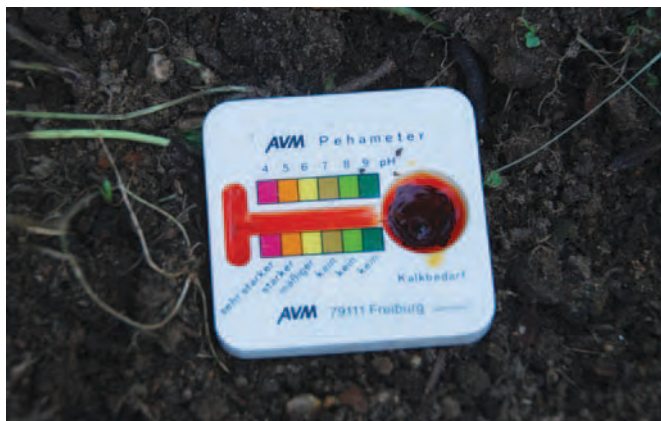
Photo 7.1 A Pehameter® is a useful low-cost tool for measuring soil pH in the field.
