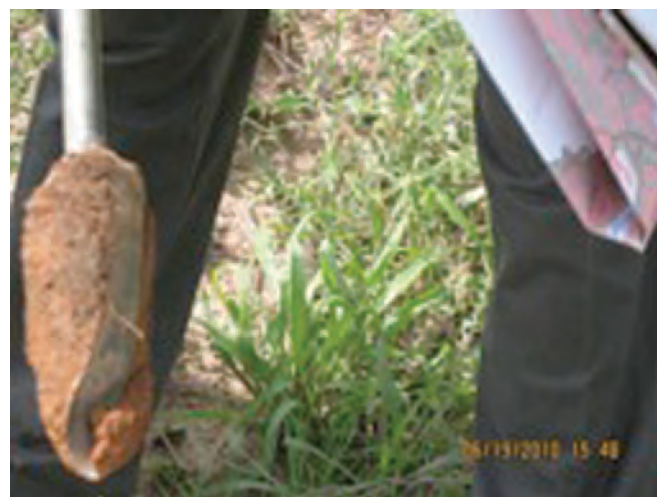
Photo 6.4 The Edelman auger is designed to sample equal amounts of soil from each depth sampled.
